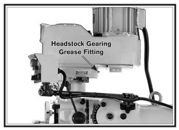
Figure 49. Headstock gearing grease fitting.
